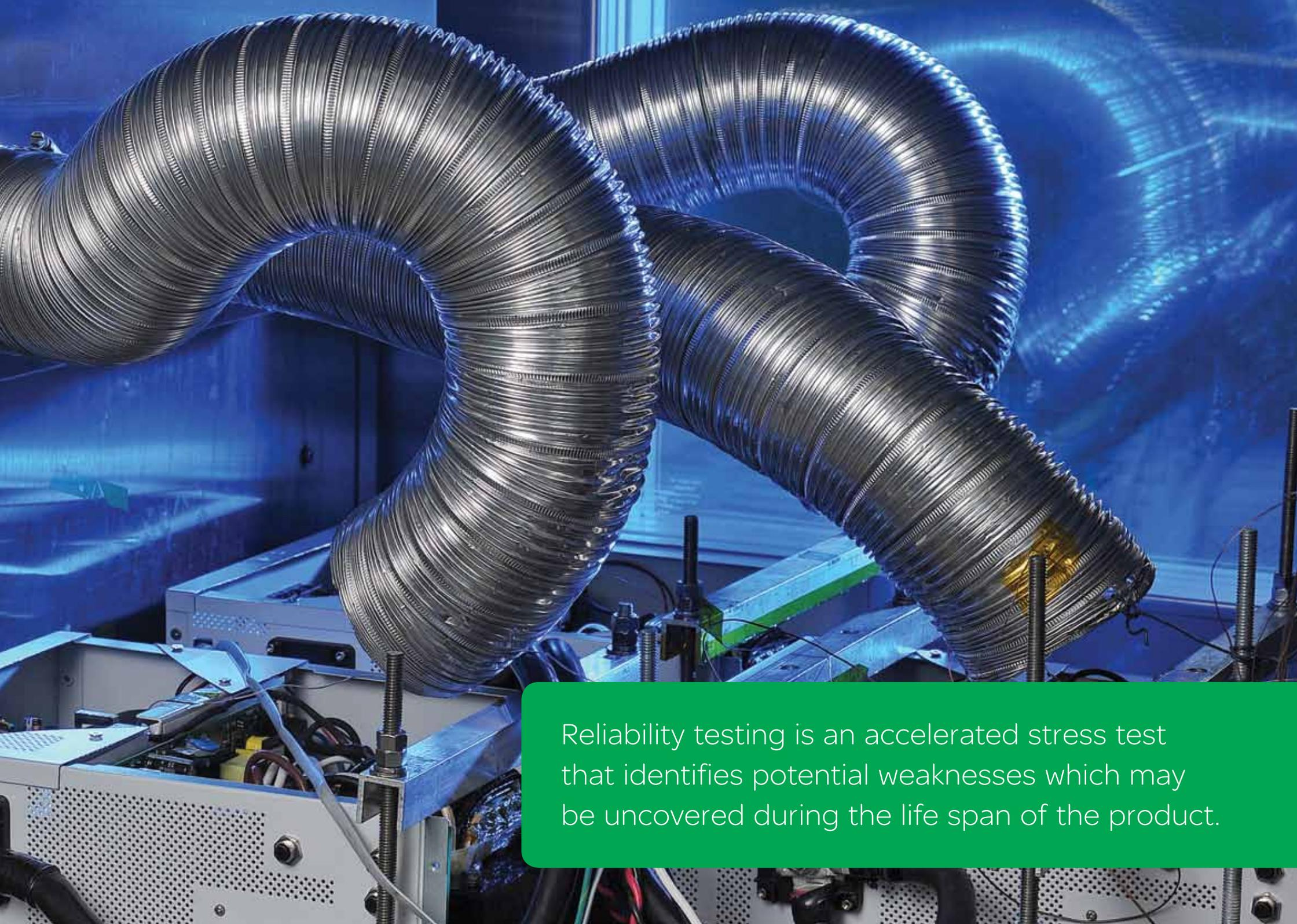
Reliability testing is an accelerated stress test that identifies potential weaknesses which may be uncovered during the life span of the product.
